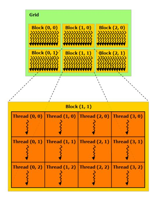
The picture above (taken from the CUDA C Programming Guide, published by NVIDIA) shows a grid (in green) of blocks. Each block contains some number of threads, and the blocks are arranged to form a *grid* covering the entire domain. In our example, we had a grid of threads of size 1024x1024. To cover this with blocks of size 16x16, we would need a 64x64 grid of blocks.
